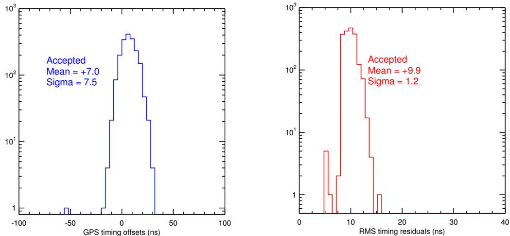
**Figure 1.** GPS receiver timing offsets and residuals as calibrated in the laboratory for all receivers to be used in the array. The vast majority of the receivers are calibrated with statistical residuals better than 15 ns.
